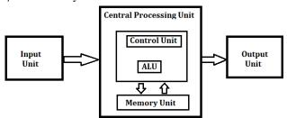
The **central processing unit (CPU)** is the brain of your computer. It handles all the instructions you give your computer. **The control unit (CU)** is a component of a computer's central processing unit (CPU) that directs operation of the processor. It tells the computer's memory, arithmetic/logic unit and input and output devices how to respond to a program's instructions.
